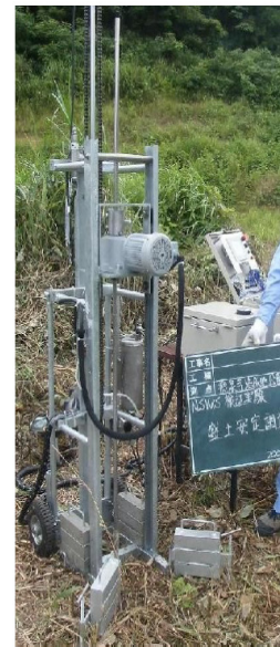
Figure 1. Externals of NSWS (Nippon Screw Weight System) testing machine
