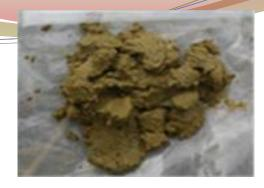
GL-3.2m Sandy silt GL-3.4m gravels mixed silty sand Detection of self-scuttling by abrupt change of penetration speed
